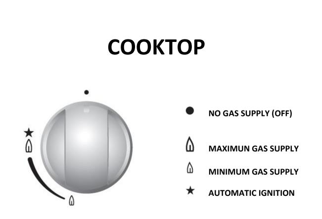
The automatic ignition means that you can operate the burners by using the control buttons only.
